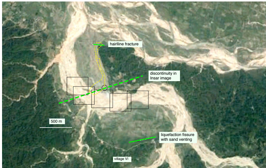
Figure M12. Close up of inset region shown in Figure M11 consists of a 2-km-wide, anastomosing river channel with fields of agriculture near its edges leading to forested slopes of hummocky Siwalik hills. The approximate path of the InSAR discontinuity is shown by a green dashed line. Black circle is landing spot for helicopter. Cracks identified by villagers shown as solid lines. Black squares approximate locations of high resolution images of river bed used unsuccessfully to locate fissures. Yellow dashed line region inspected on foot.
